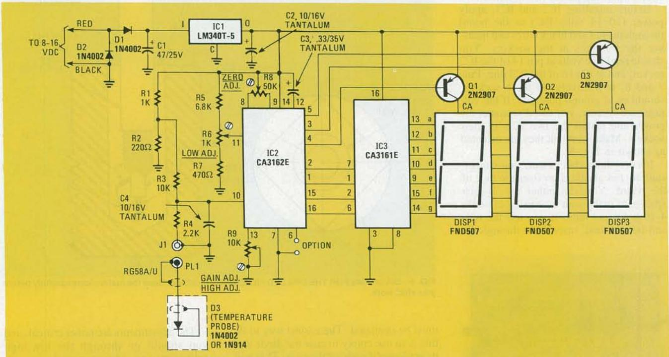
FIG. 1—THE BASIC DIGITAL TEMPERATURE GAUGE consists of a probe, an A/D converter (IC2), a 7-segment LED decoder/driver (IC3) and, of course, the display LED's themselves.
