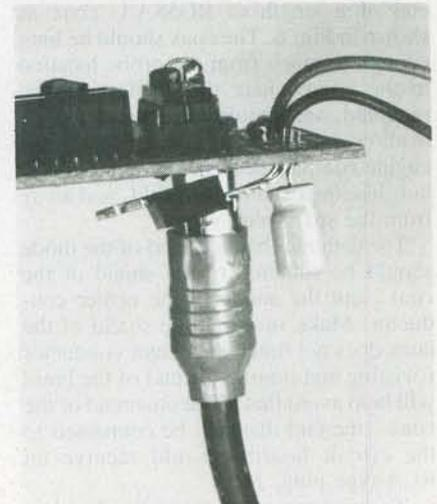
FIG. 4—BEND IC1 OVER BACKWARD on the bottom of the board as shown.
