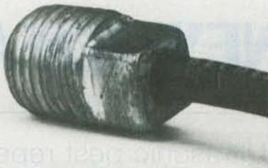
FIG. 7—COMPLETED FILLER-BOLT probe with cable attached.
