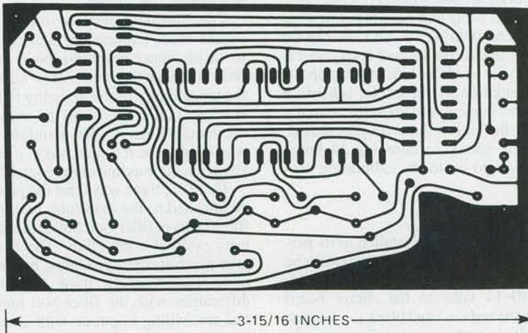
FIG. 2—YOU CAN ETCH this single-sided PC board yourself, or buy it from the source indicated in the Parts List.
